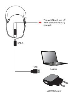
Charge from USB AC charger or laptop (NOTE: No data signal when connected to laptop, only for charge).
